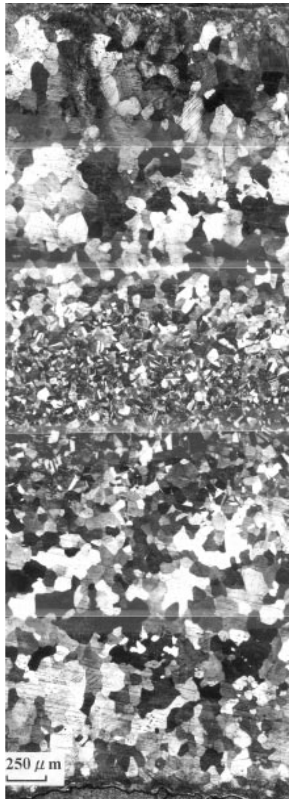
Fig. 3 Microstructure (grain structure) of as-cast phosphor bronze strip produced by the twin roll caster with the following casting conditions: setback = 80 mm, casting speed = 15 m/min, roll gap = 4.5 mm, roll separating force = 1 ton, and pouring temperature = 1065 °C
