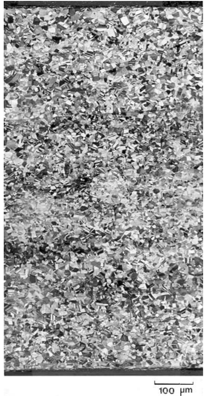
Fig. 8 Microstructure of as-annealed phosphor bronze sheet produced by twin roll casting after cold rolling and annealing at 550 °C for 1 h
